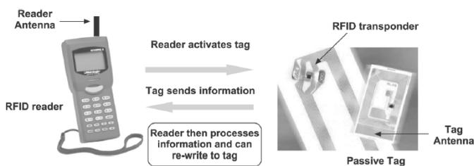
Figure 4 - RFID reader and tag communication flow diagram.
